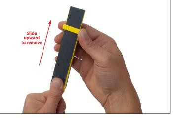
Cut a piece of sandpaper that is approximately 1" wide by 11" long. Fold the strip in half and place it over the top of the Slide sanding file as shown here. Start downward sliding the sliding lock downward
