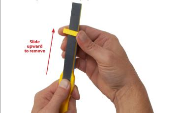
Cut a piece of sandpaper that is approximately 5/8" wide by 11" long. Fold the strip in half and place it over the top of the sanding file as shown here. Start sliding the sliding lock downward **Large Flat File Sander**
